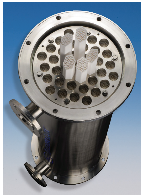
Figure 6: The Membralox 36P48-40HCB module consists of 36 EP48-40IC multi-channel membranes, mounted in a compact Membralox HCB housing.
